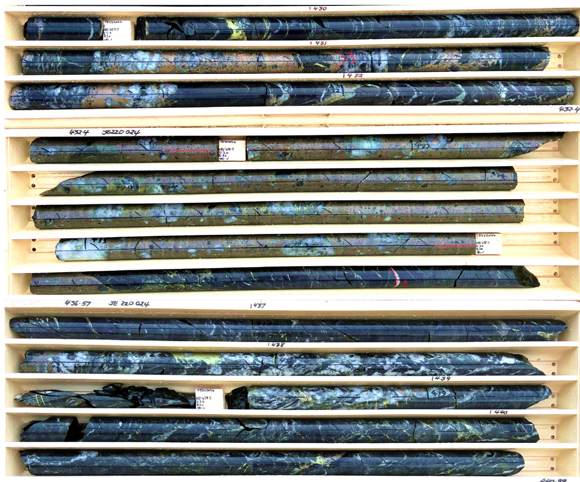
Figure 8: J1 Lode Extension drill hole JE22D024 in the Matilda shoot showing massive and semi-massive sulphide mineralisation with abundant chalcopyrite (yellow) from 430-441m.
