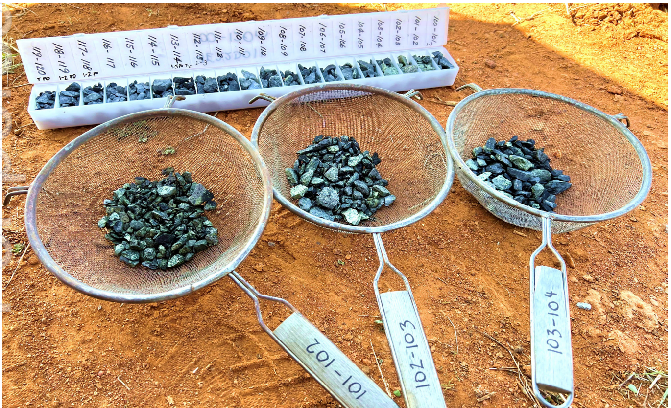
Figure 5: J1 Lode Infill RC hole JE22D011 drill chips from 101-104m with massive and semi-massive sulphide mineralisation – copper sulphide (chalcopyrite) is yellow.
